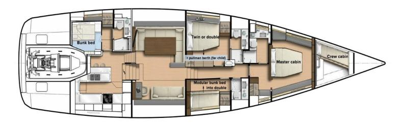
23,17 m Length over all 6,10 m Beam 45,000kg **Displacement**
