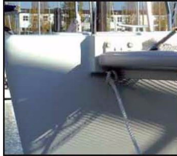
ATTACH THE BRIDLE TO THE FORWARD BEAM
