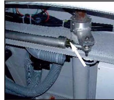
CABLE TENSION SYSTEM
