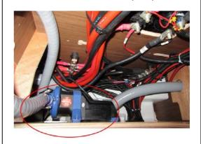
NOTE: The valve must be opened before starting the pump.
