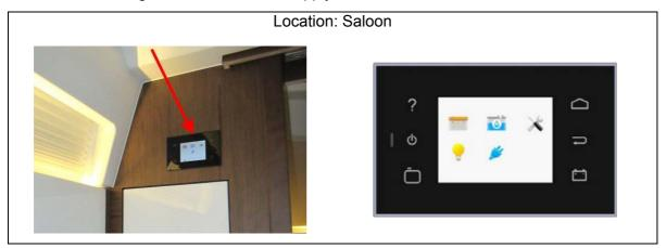
The screen NAVICOLOR is a touch interface for viewing and controlling the auxiliary functions of the boat:
