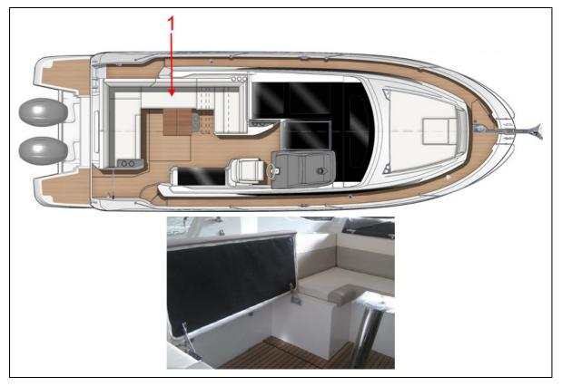
The liferaft (not supplied) must be stored in the space provided for it (Ref 1). A pictogram allows for easy location.
