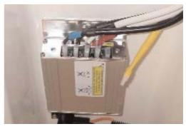
The yellow wire (engine DC supply) can be disconnected manually by accessing the connection box.
