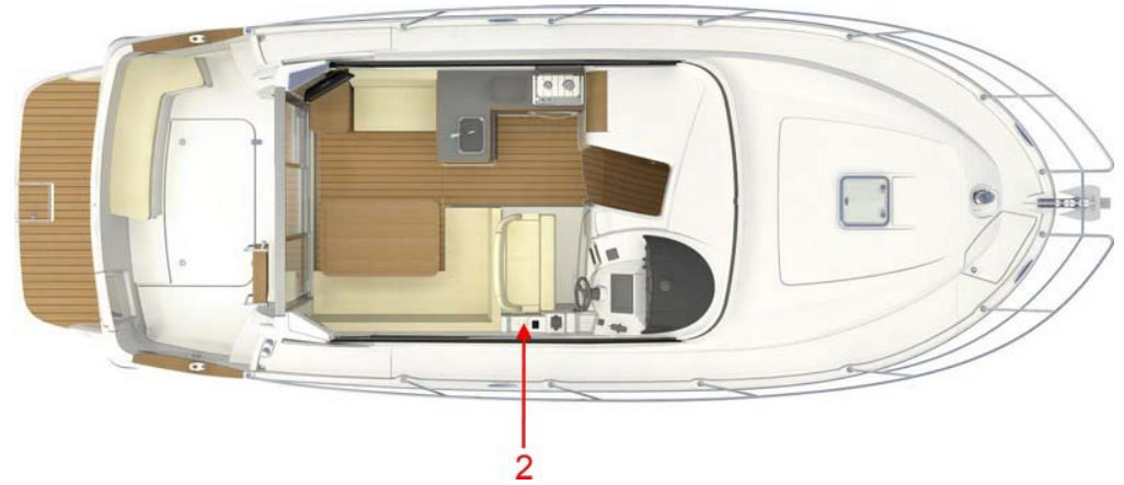
Ref 2: Remote pull switches Location: Steering station
