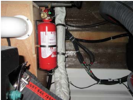
Ref 1: Fixed extinguisher Location: Engine compartment
