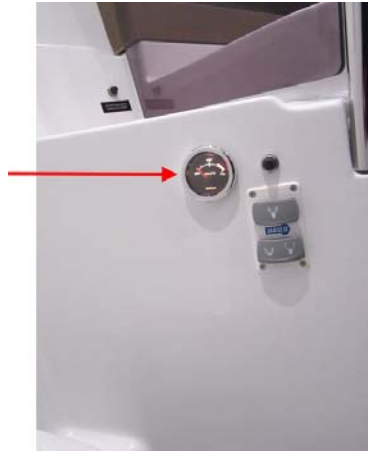
Black water tank gauge Location: Head
