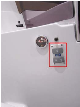
Electric toilet control
